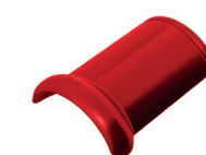
1. Thai Ridge Use to form the top angle and the angle hip areas (3.3Pcs./1 Meter long)
